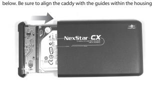
4-3 Secure the caddy to the housing using the screws provided.
